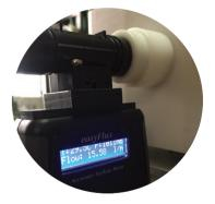
Adjust the flow rate up to reach the desired value in the display of easyFlux. in easySPT100 by using the button - and + on the rear user interface. In the easySPT200 by using a screw driver to rotate the flow rate screw under the nozzle.
