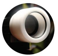
Check the nozzle adaptor and clean it from dust. Check also that the sealing O-Ring is in palce. That's important to avoid lost in flow and to maintain attached the easyFlow to the instrument.
